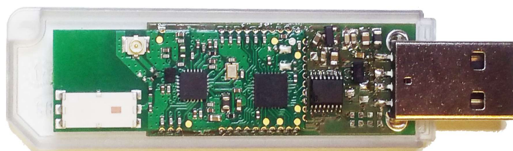
Figure 6: Evaluation board as USB Dongle with housing
