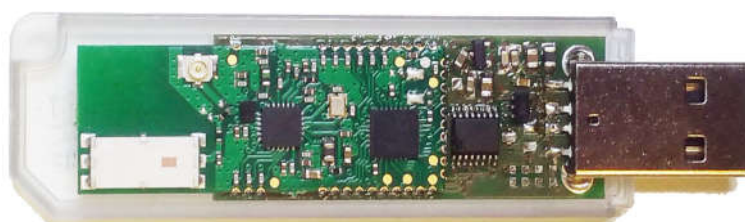
Figure 6: Evaluation board as USB Dongle with housing
